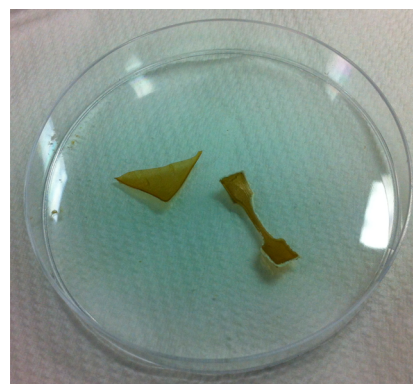
Figure 8. Films prepared from dissolved feather in [DMEA][HCOO].
